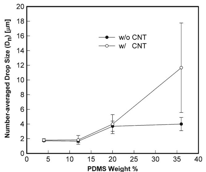
**Fig. 5** Comparison of the number averaged-drop size of blends and CNT blend dispersions
