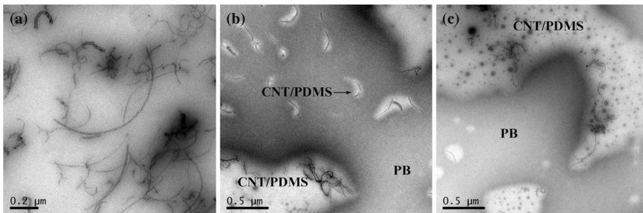
**Fig. 6** Cryo-TEM images of CNT master (a) and B12CNT025 (b, c)
