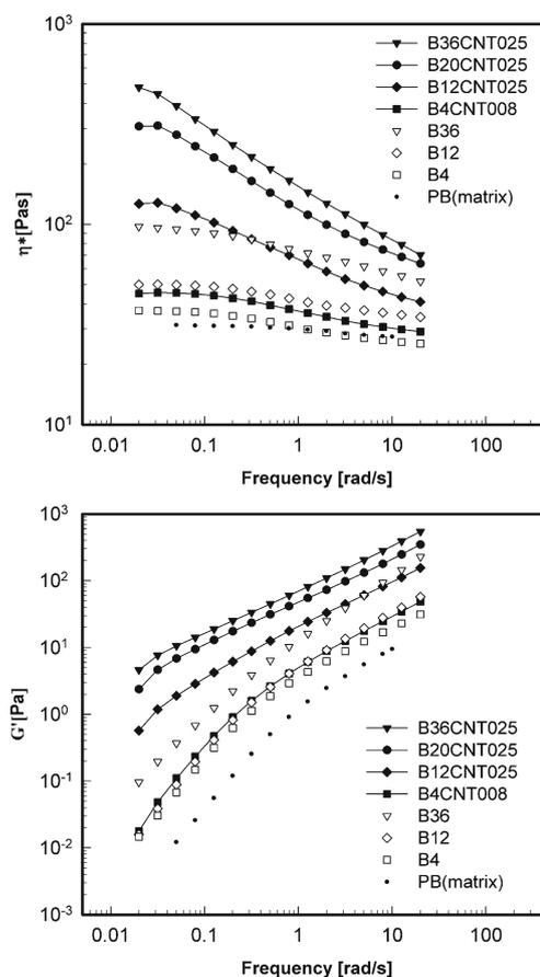
**Fig. 3** Rheological properties of blends and CNT blend dispersions: complex viscosity (a) and storage modulus (b)
