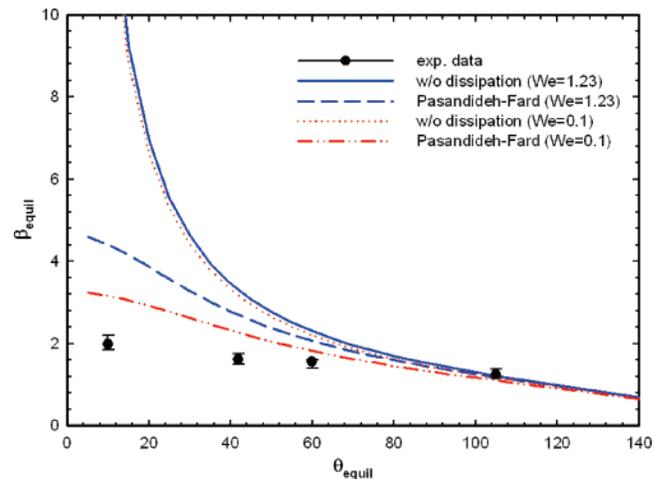
**Figure 11.** Measured maximum spreading values compared with the model predictions. Experimental values were obtained for various  $We$  values between 0.1 and 1.23. The deviations become large for small contact angles. This difference appears to be the result of the large viscous dissipation near the contact line.
