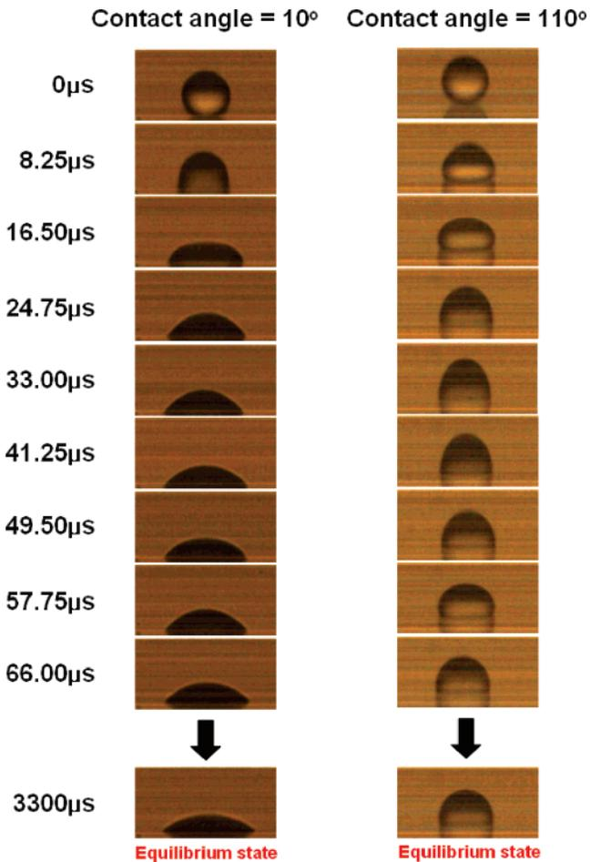
**Figure 7.** Drop impact dynamics on two different surfaces with contact angles of 10 and 110° at the same impact condition as in Figure 6. The drop deformation after the impact differs significantly. The drops take spherical shapes at the equilibrium state regardless of contact angle.
