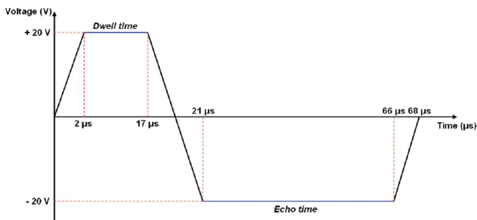
**Figure 2.** A typical voltage wave form used in the experiment.
