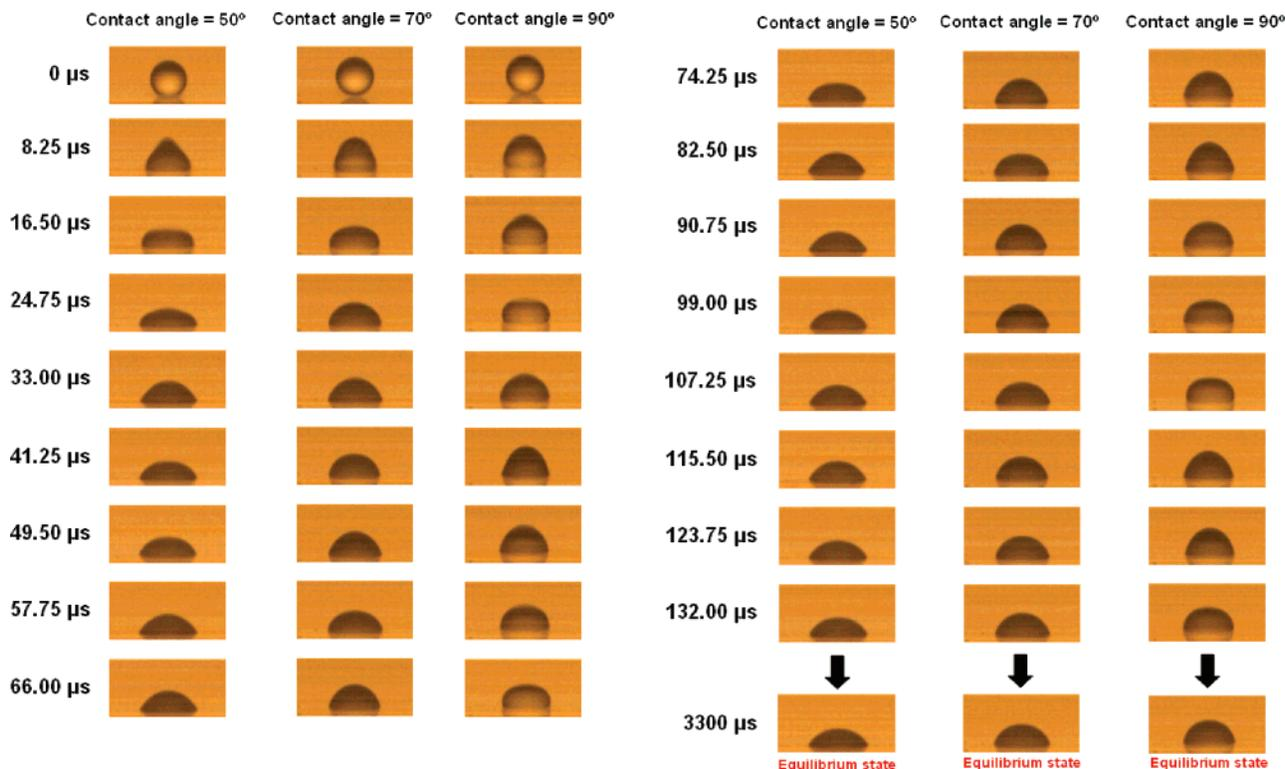
**Figure 6.** Drop impact dynamics on three different surfaces with contact angles of 50, 70, and 90° when  $We = 1.23$  and  $Oh = 0.017$ . Depending on the wettability of surface, the drop deformation after the impact changes significantly. However, no lamella is formed. There are oscillations along the vertical and horizontal directions.
