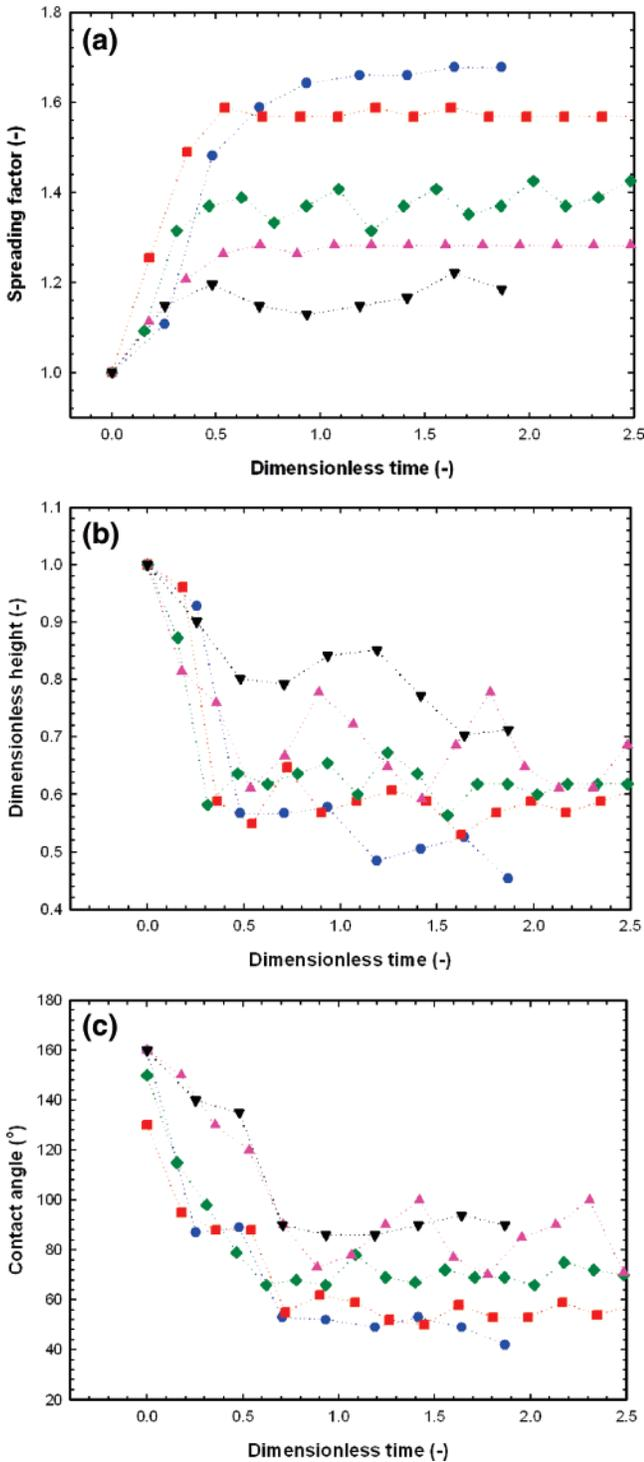
**Figure 9.** Changes of the maximum spreading (a), drop height (b), and contact angle (c) with dimensionless time. The dimensionless time is made from the inertial time ( $tU/D$ ). After the initially fast changes, the drops oscillate with a period comparable to the time scale. The diameter and height take the equilibrium values after several oscillations. (●: contact angle = 10°; ■: contact angle = 50°; ◆: contact angle = 70°; ▲: contact angle = 90°; ▼: contact angle = 110°).
