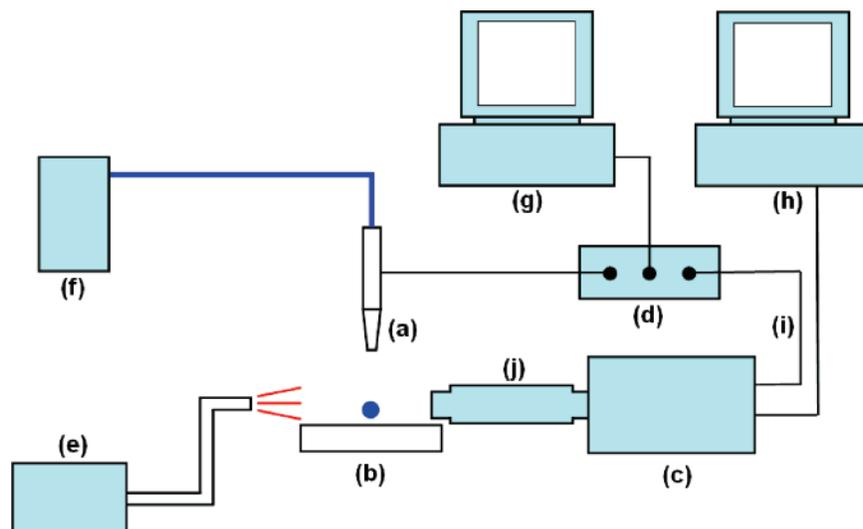
**Figure 1.** Schematic diagram of the experimental setup: (a) inkjet nozzle; (b) solid substrate with controlled contact angle; (c) high-speed camera; (d) jetting driver; (e) illumination source; (f) pneumatic system; (g) jetting control computer; (h) image processing computer; (i) triggering; (j) objective lens.
