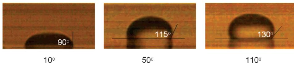
**Figure 8.** The contact angle values when the drop takes the maximum diameter of the wetted area (the maximum spreading condition). The contact angle values are not the same and increase with the static contact angle.
