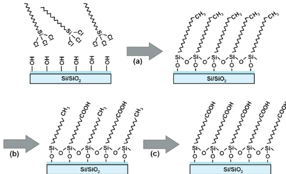
**Figure 3.** Procedure for controlling the contact angle of a glass surface. A hydrophobic self-assembled monolayer is adsorbed and then treated with UV–ozone to control the hydrophilicity by varying the exposure time: (a) adsorption and reorientation of SAMs; (b) UV–ozone plasma treatment for partial oxidation; (c) extended UV–ozone treatment to increase the wettability.
