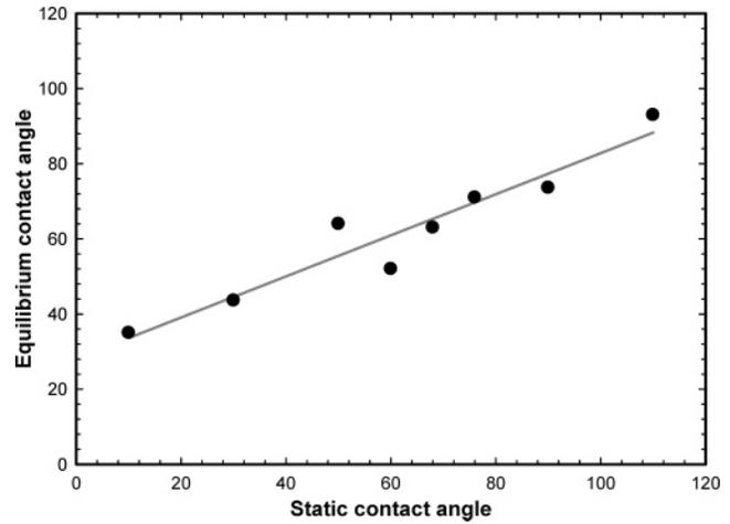
**Figure 10.** The equilibrium contact angle after the impact vs the static contact angle. When the static contact angle is small, the contact line stops before the contact angle reaches the static value. This is caused by the viscous dissipation during spreading. For large static contact angles, the equilibrium angle is smaller than the static angle as a result of the receding motion during oscillation.
