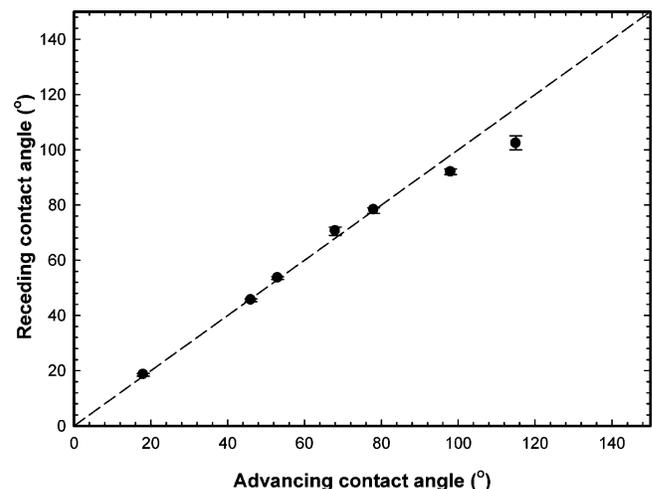
**Figure 5.** Receding vs advancing contact angle values. In this case, the two values are almost the same. The diagonal line is for guiding the eyes.
