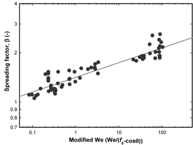
**Figure 12.** Spreading factor vs the modified Weber number based on the impacts on different surfaces with different velocities. The spreading factor ( $\beta$ ) is well correlated with the relationship  $\ln \beta = 0.090 \ln We' + 0.151$ , with  $r^2 = 0.846$ .
